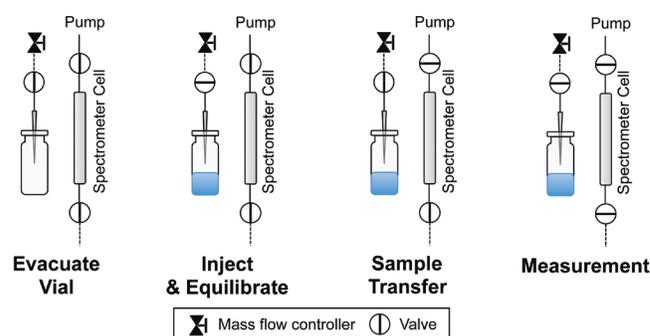
Fig 1: Mass flow control sample transfer.
